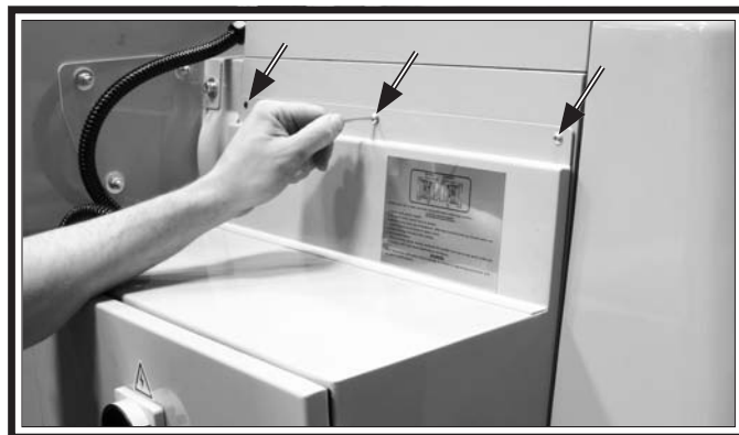
Figure 122. Removing electrical cabinet fasteners.
